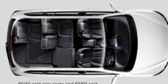
60/40 split rear seats and 50/50 split third row seats allow alternate 5 seat configuration
